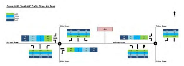
Figure 3-4 AM peak "No build" scenario traffic flow (2030)
