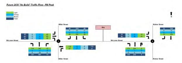
Figure 3-5 PM peak **"No build"** traffic flow (2030)
